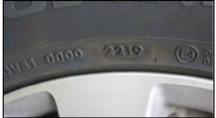
Date code of 2219 means week 22 (June) of '19; is less than 2 years old
