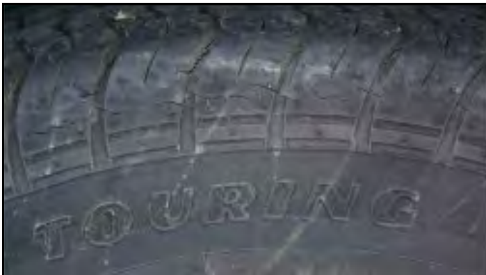
Cracks in sidewall and tread mean this tire's life is over
