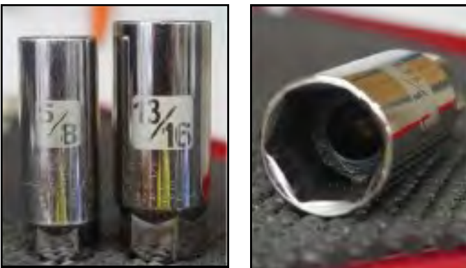
Spark plug sockets in 5/8" & 13/16" sizes; rubber insert
