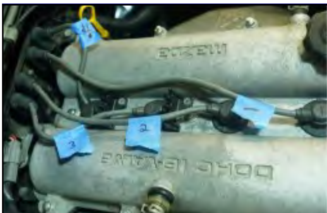
Plug cables labeled with masking tape before removal
