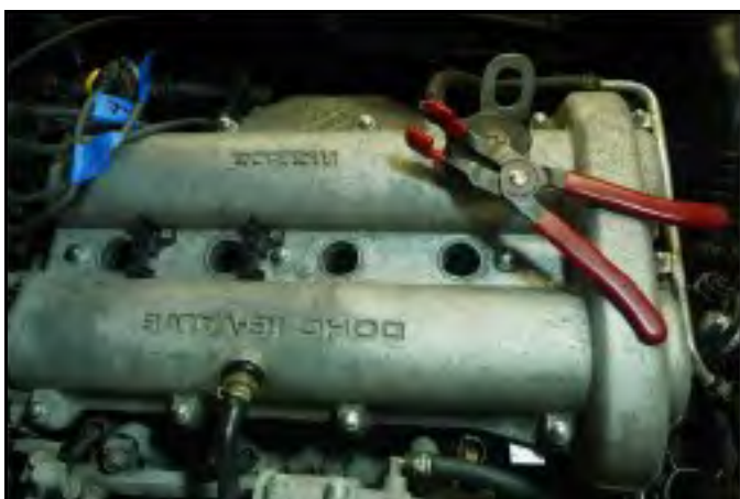
Pliers made for spark plug cables make removing them easier
