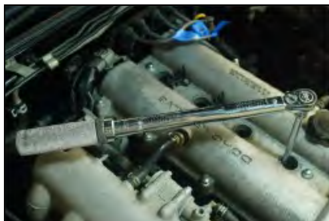
You will never incorrectly tighten a plug if you use a torque wrench
