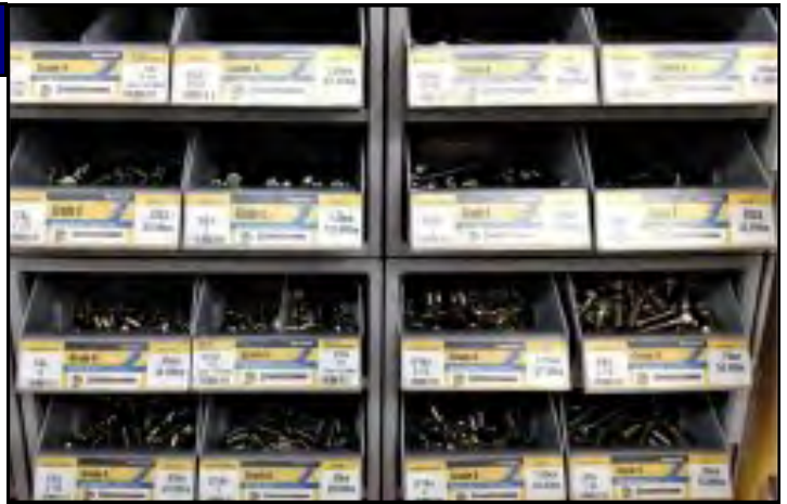
U.S. Grade 8 hardware in various sizes [diameter x length]. Thread pitch is indicated as "coarse".
