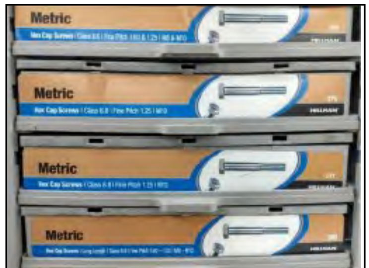
Metric hardware, Class 8.8 hardness, diameters M8, M10, & M12, thread pitches 1.00 & 1.2
