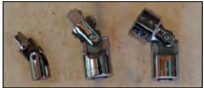
U-joint extensions are available as ¼", 3/8" and ½" drive as well as sockets
