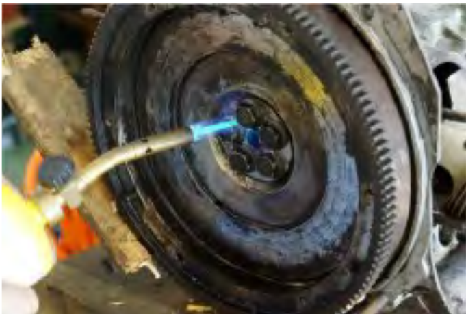
To break these bolts loose, heat is aimed at flywheel,
