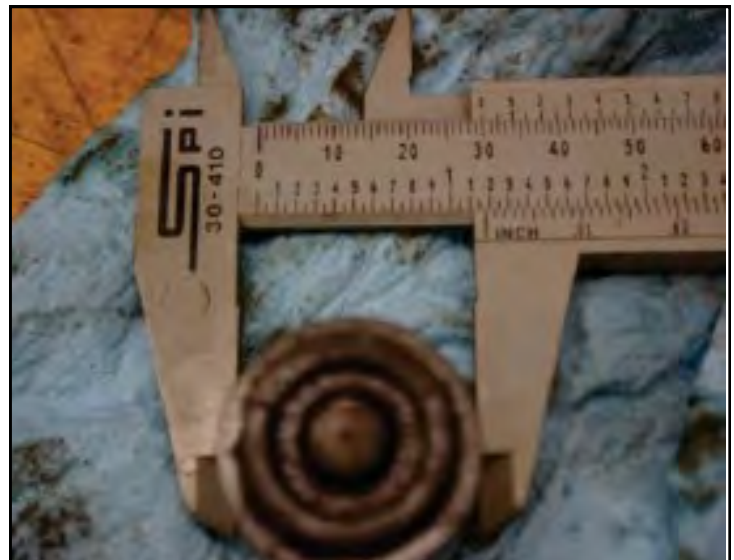
Above: using outside diameter jaws, vernier calipers confirm brake caliper piston diameter is 30mm
