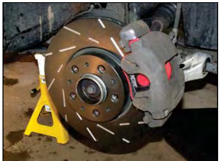
the new brake pads in red are mounted within this floating caliper
