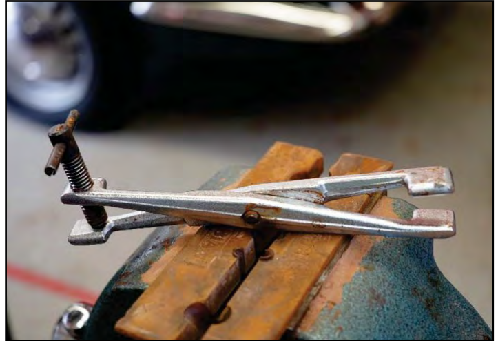
My old and simple caliper piston spreader
