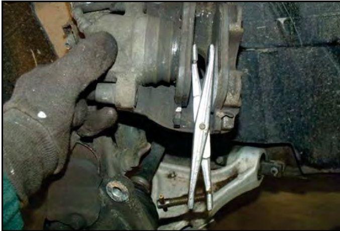
The tool at work. Note placement of worn pad on each side to provide a pushing surface.
