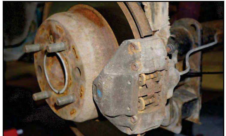
With a fixed caliper like this, just undo its bolt and swing it away from the rotor. Do not disconnect the brake line!
