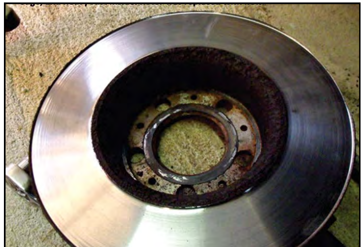
While rotor contact surface looks smooth, note lip on outer edge, and heavy rust inside. Rotor was replaced with new.
