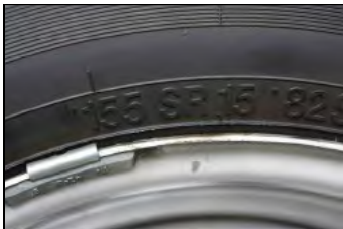
When no aspect ratio is shown, like this 155SR15 tire, it is presumed to be "80". S" is a speed rating.
