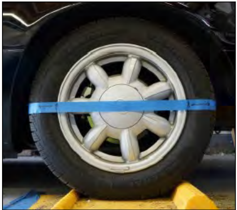
Overall diameter equals sidewall height times two, plus wheel diameter
