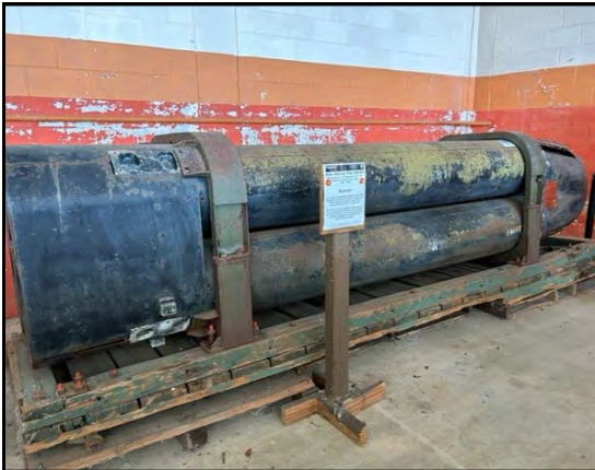
Booster Four solid rocket motors propel the Nike Hercules missile at incredible speed. The solid fuel is laid down in layers and burns evenly from the inside out.
