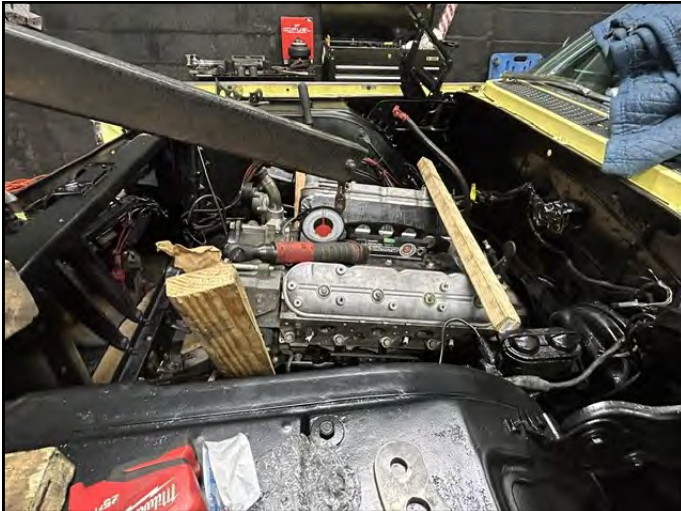
Engine installation aided by inserting wood to stabilize it
