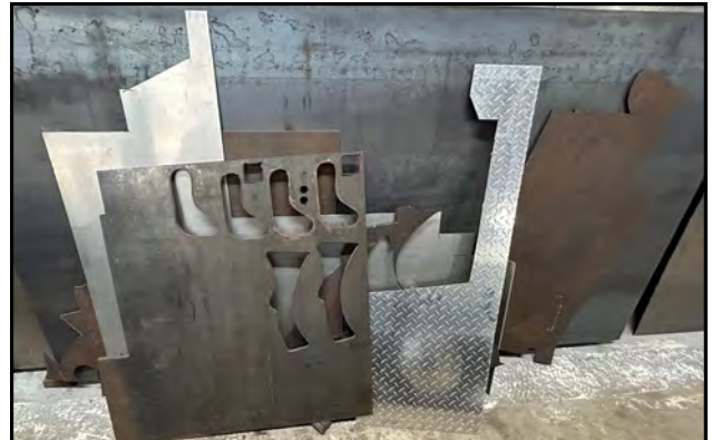
Different metals are used for making templates or replacing damaged metal in floors, quarters, etc..
