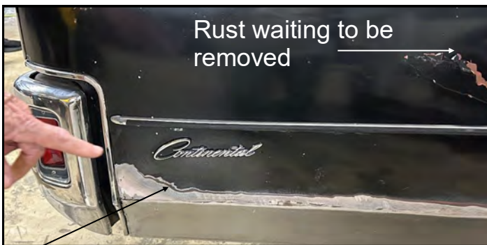
Rust was removed by grinding down to bare metal.
